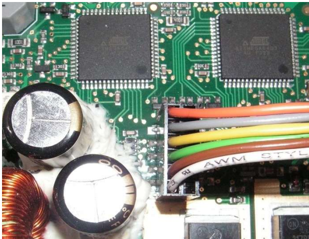
Mounting of 6-wire cable for Power input PCB on main-unit PCB.
